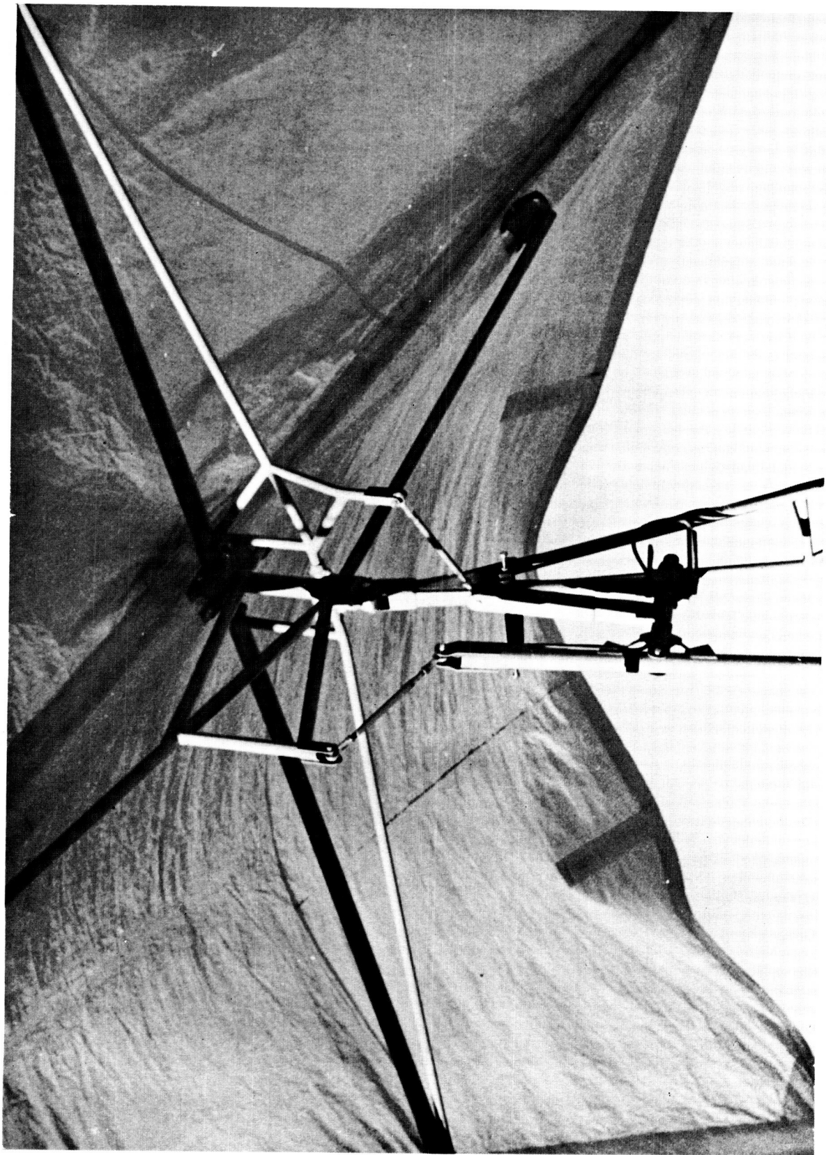
Figure 5.- Photograph of control linkage used on vehicle A.
